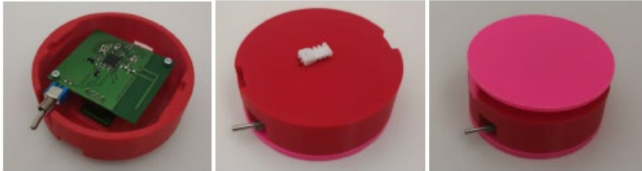
Figure 8: Our sensor at different stages of assembly
